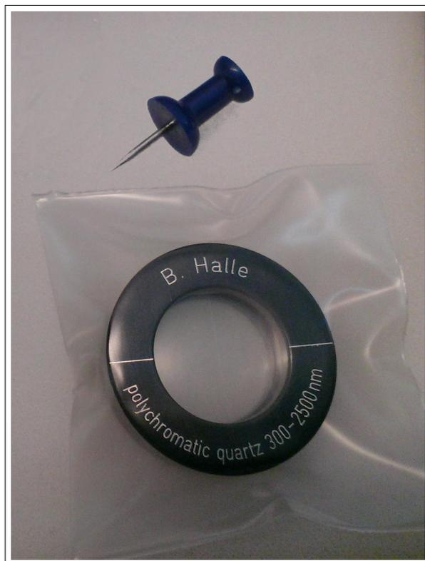
Figure 1. The manufactured polychromatic modulator for the 300–2500 nm wavelength range.
