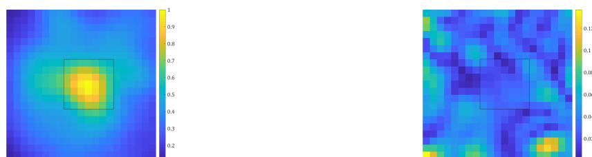
Fig. 2: s_0 of an Eutelsat 172B image (left) and its DoLP (right). The square indicates the low noise region.
