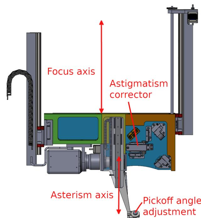
Figure 5. Mechanisms overview in a single LWFS.
