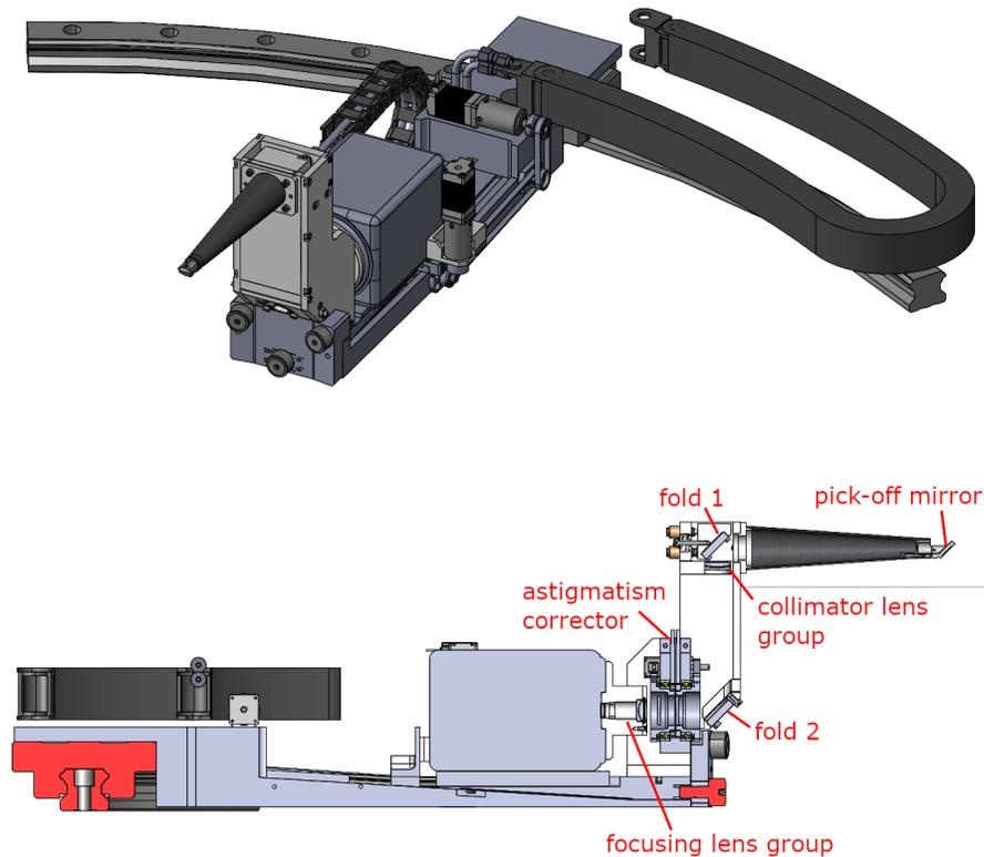
Figure 8. NWFS unit: isometric view (top) and section view (bottom).
