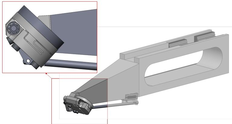
Figure 7. LWFS pick-off mirror mechanisms showing cam actuation.
