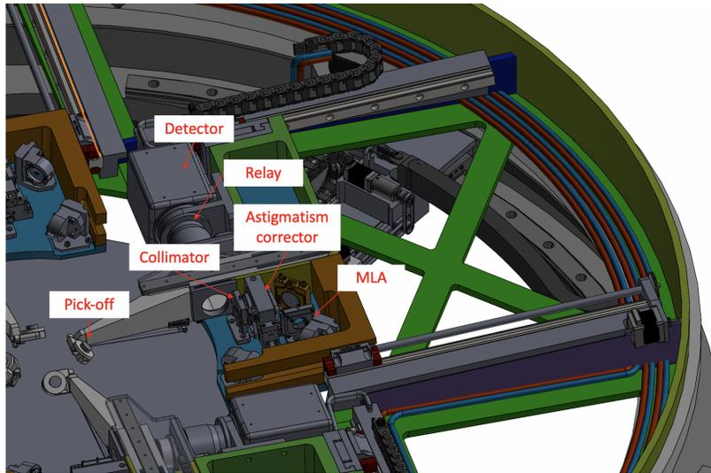
Figure 4. Overview of a single Laser Guide Star WFS (LWFS) mounted on the LGS WFS sub-assembly.
