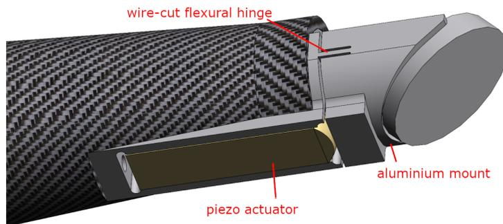
Figure 9. NWFS pick-off mirror mount showing the mechanism hinge.
