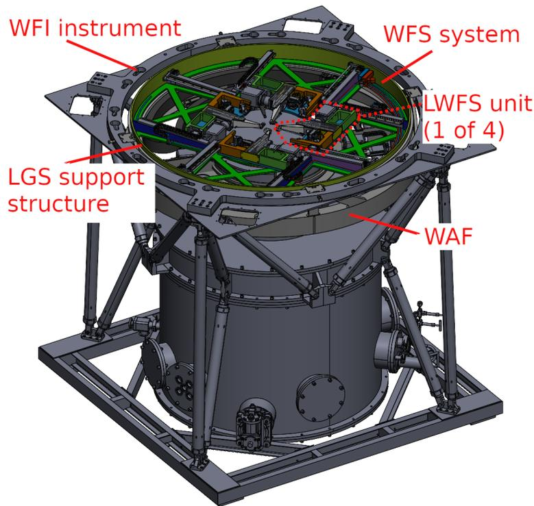
Figure 2. Cassegrain Wavefront Sensor system preliminary mechanical design, including the Wide Field Imager (WFI) instrument preliminary design. The WFS model is provided by Sumitomo Heavy Industries and OptCraft in Japan.
