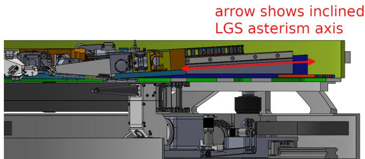
Figure 6. The LWFS pick-off mirror traces a cone to accommodate the curvature in the telescope focal plane.
