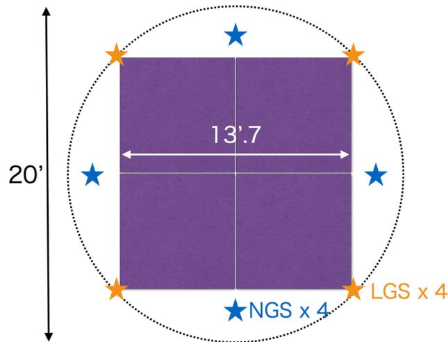
Figure 1. GLAO Laser Guide Star and Natural Guide Star asterisms at the Cassegrain focus; the purple square represents the science field of view.
