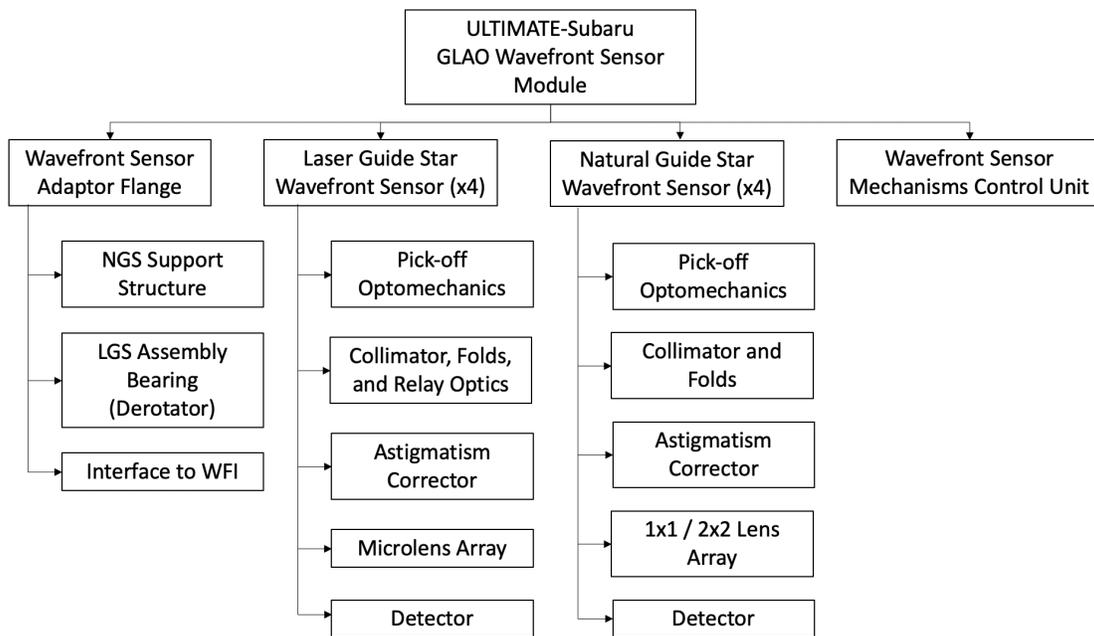
Figure 3. GLAO Wavefront Sensor Module Architecture
